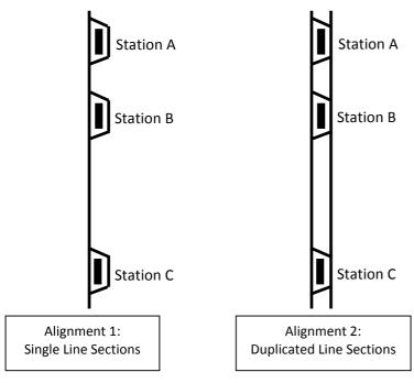
Figure 12: Single and Duplicated line sections
