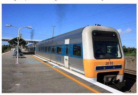
Figure 23: Two-car Endeavour set (used in the Hunter Region of NSW)
