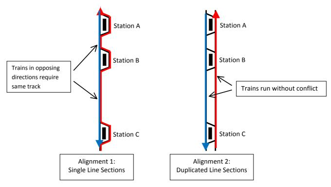
Figure 2: Train routing on single and duplicated track
