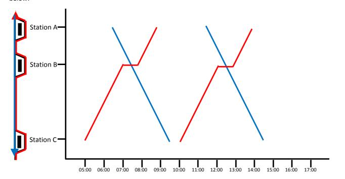
Figure 5: Example schedule on single line sections
